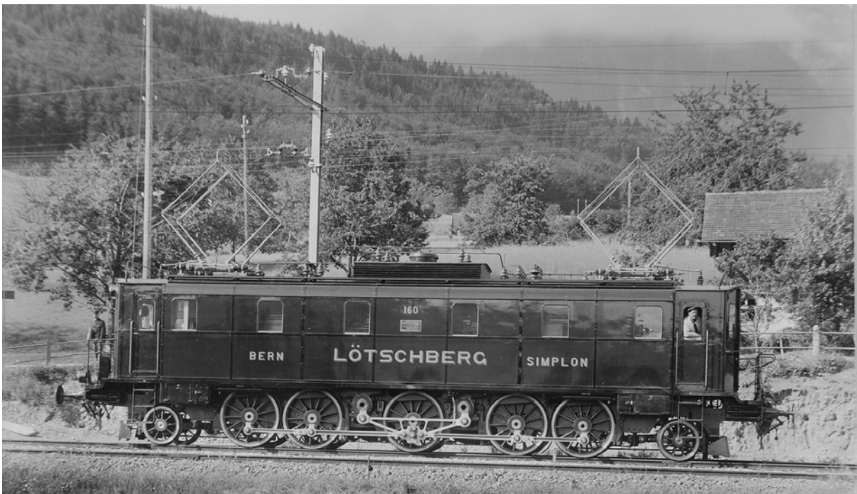
Figure 11 – Be 5/7 electrical locomotive developed for BLS (1915)
