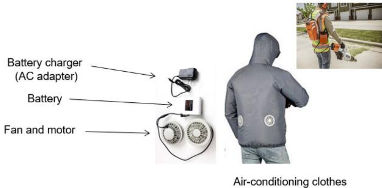
Figure 2 – Example of Separable battery pack
