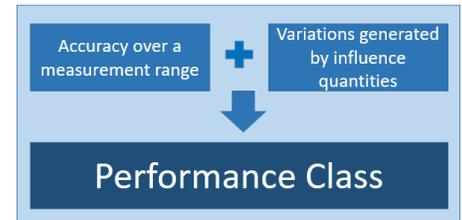
A **performance class** is an essential characteristic that enables measurement performance levels of PMDs from different manufacturers to be compared. It ensures that users can rely on the quality of the measurements of their PMD subjected to the severe constraints of an electrical installation.
